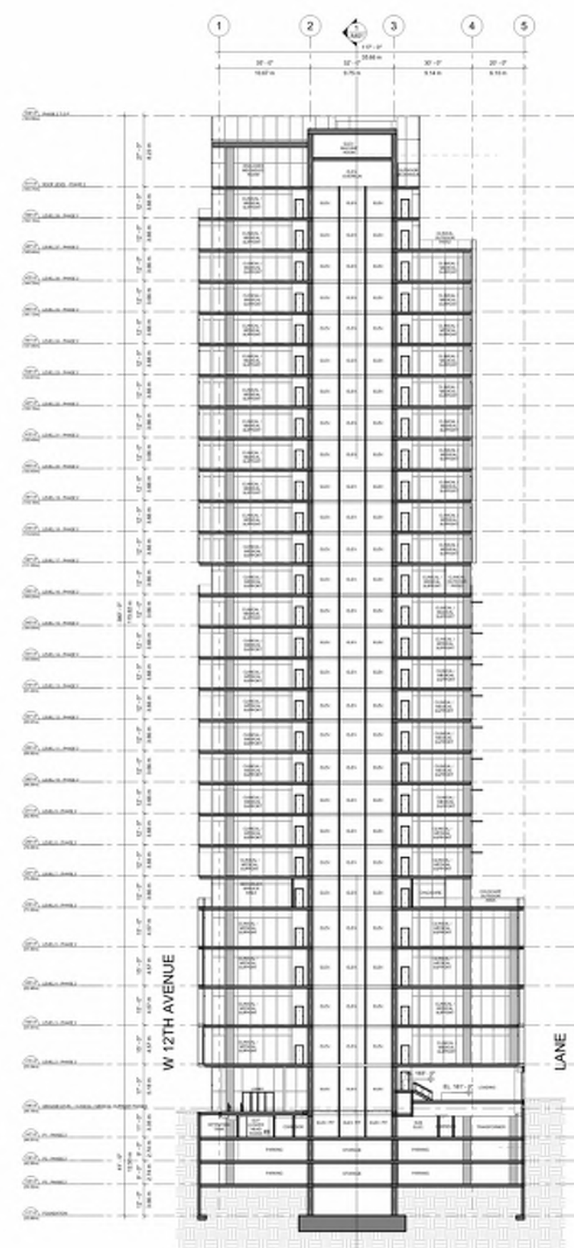
66 CROSS SECTION THROUGH CLINICAL SUPPORT CORE PHASE 2 SCALE: 1/8" = 1'-0"
